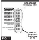
To program your BirdXPeller PRO unit you will need a small screwdriver, toothpick, or other pointed, rigid object to move the switches in the switch array (see FIG. 1). The switch arrays are the switch banks
