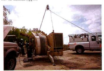
According to Condux national accounts manager Ernie Neilsen, the Xcel conductor installation project called for a specific piece of equipment. Neilsen said, "Because we needed to meet strict conductor handling requirements and wanted to minimize any environmental impact on the right-of-way, we had to make sure we selected the right puller-tensioner for the job. In this case it was two AFB 506 puller-tensioners."
