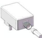
**Plug attachment:** Firmly attach the plug (supplied separately) to the unit's power cord by screwing it onto the screw-threaded attachment at the end of the cord – see diagram. When attaching the plug for the first time, make sure the 2 pin plug is the right way round. Match 'flat' and 'keyway' for proper contact. Check before tightening, as the fit only works in one direction. \*\* Use only the plug and power adapter supplied with the unit.
