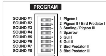
The Sound Setting Switches are the first eight switches in the switch array, to set the sonic (audio) sounds only.
