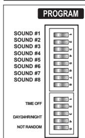
To program your BB-PRO unit you will need a small screwdriver, toothpick, or other small, rigid object to move the switches in the switch array. The switch array is the switch bank located in the top left corner of the unit (under "PROGRAM"). **A switch is ON if the switch is moved to the right-hand side. The switch is OFF if the switch is moved to the left-hand side.**
